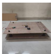
Fig.no. 3.6.4 Vibration table with attach motor and sensor
